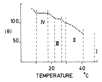
Figure I - Variation of  $|\Theta|$  the phase retardation between the ordinary and extra-ordinary ray of polarized light as a function of temperature.  $|\Theta|$  Represents the magnitude of the retardation where the sign was found negative, a result of negative birefringence. Sample composition was 40% MTABS and 60%  $D_20$ .
