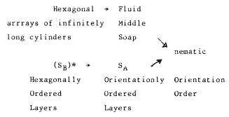
)\* indicates that although the hexagonal and  $S_{\mbox{\footnotesize{B}}}$  have some similarities such as optically uniaxiallily and rigidity, the two structures are not necessarily equivalent.
